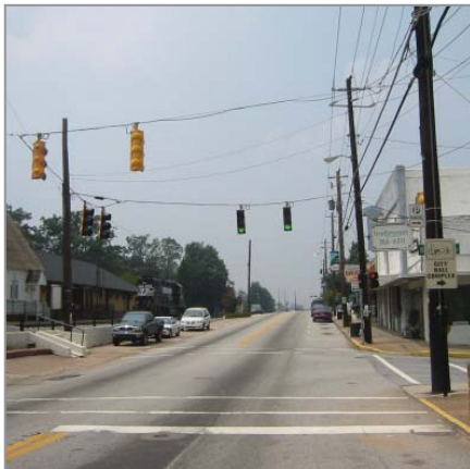
Pedestrian crossings along North Central Avenue are poorly marked
