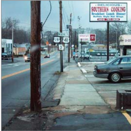
Excessive curb cuts compromise sidewalks on Dogwood Drive
